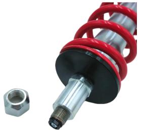
On the other side, the upper fixation come through the top mount car. Tight-up the 27mm nut with an impact wrench.
