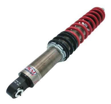
The rear damper do not use strut. Damper fit in the car by ball joint bearing.
