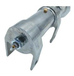
Then, screw the nut and the locknut to the rod. If the rod turns around the strut, use a 10 flat wrench on the rod to tighten the nut. Unscrew the 3mm hexagonal screw inside the rod and let it exceed from the rod.
