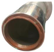
The damper come to the strut trough a wiper seal. To protect the seal during assembly it must be grease. Guide ring into the strut must be grease too.
