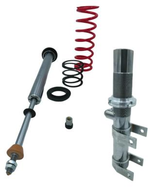
The front damper assembly is composed of the damper and a strut. Damper assembly can be purchased without the strut.
