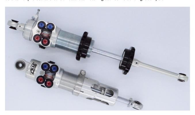
These dampers are delivered with an externally adjustable Blow Off system that help for the kerb crossing and optimizes the recovery of grip after it. This system also increases the overall comfort in the vehicle, which is not insignificant in terms of human and machine reliability in endurance events.
