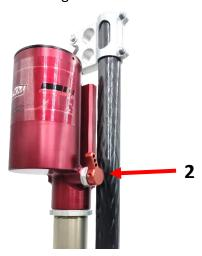
For the first 30°, you can set the down speed. The jack is pressurized, that means the rod will automatically go in the tube. You will not have any free stroke after turning out the releasing button. Be careful, don't trap your hand with the jack pad, it will come fast. If you want to retract the jack correctly, put the pin on the tube before closing the scroll wheel 2.
