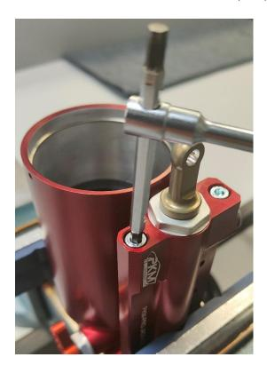
Disassemble the pump from the body. Unscrew the piston from the tube.
