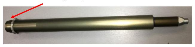
Remove the circlip and take of the separator piston from the body. Screw **OT-EXT-002-A** into the separator piston to get it out.
