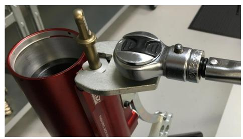
Set the tap assembly into the body. Screw the cap JA-BOU-018-A tap into the body with Loctite 243 at 20N.m TOOOl. Screw the rod JA-TIG-009-B at the maximum to close the tap. Set the scroll wheel onto this axle at 45°. Screw HC040N006E109A with Loctite 243.
