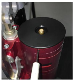
The jack is ready to be tried. Lock the jack between a scale and a fixed metal beam. Pump the jack until 700kg appears in the scale. Let the jack for 1hour and check, if the weight is the same, the jack is ready to be packed on a race car.
