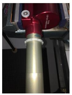
Lock the locknut JA-ECR-001-B to the body with Loctite 243 at 35N.m with OT-SER-193-A.
