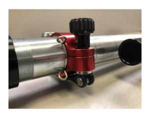
Please pay attention to place the ears of the circlip at the opposite angle of the lifting pin, as shown by the picture
