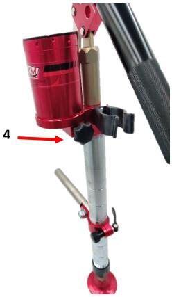
For the first 30°, you can set the down speed. The jack is pressurized, that means the rod will automatically go in the tube. You will not have any free stroke after turning out the releasing button. Be careful, don't trap your hand with the jack pad, it will come fast.
