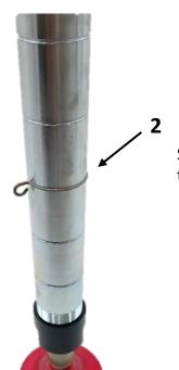
Set the circlip named 2 at the height of your car. Be careful, do not set it up to high, in case of a puncture your call will be lower.
