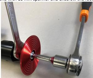
• Put the foot off, unscrew the Torx screw in the tube (don't lose the O-ring).
