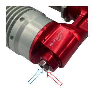
**Low Speed Bump Damping Adjuster** (blue arrow)
