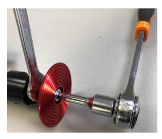
• Put the foot off, unscrew the Torx screw in the tube (don't lose the O-ring).
